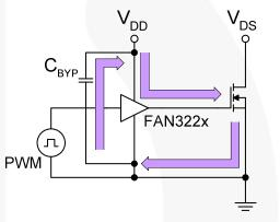
Figure 46. Current Path for MOSFET Turn-on
