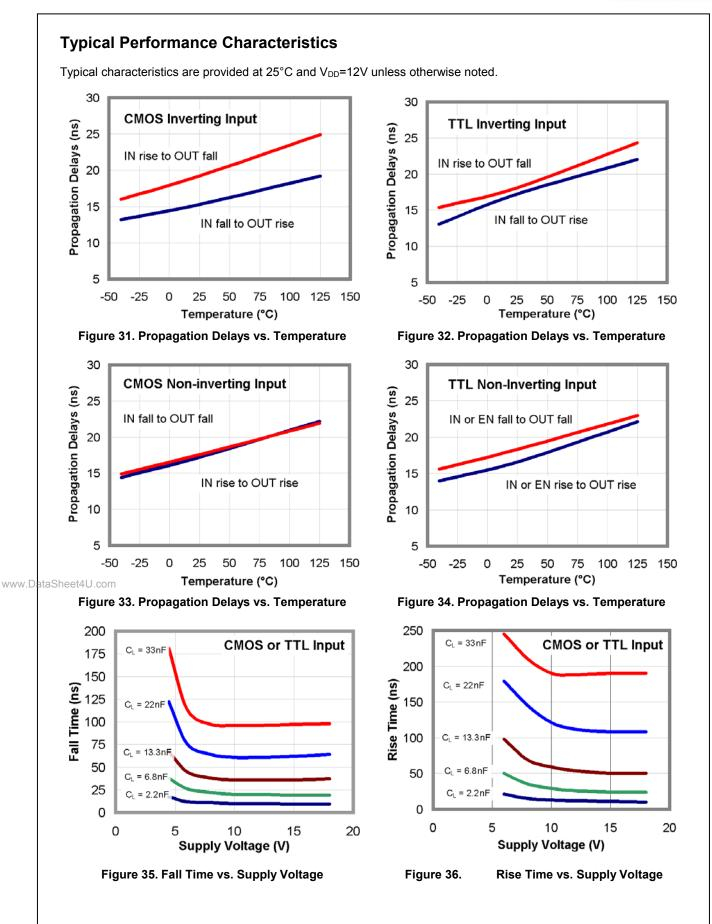
AN3223 / FAN3224 / FAN3225 — Dual 4A High-Speed, Low-Side Gate Drivers
